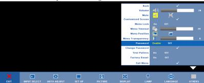
Enable the Password function will pop up a character screen, key in a 4-digit number from the screen and press the Enter button.
